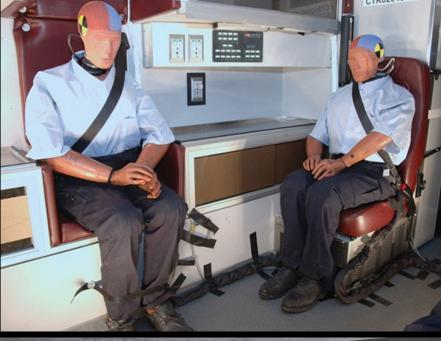
STATIC LOAD TESTS ARE PERFORMED TO TEST THE SEAT BELTS, DOOR LATCHES/HARDWARE, AND CABINETS
