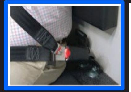
Horton's detachable threepoint harness system & barrier seat bolsters. The detachable feature on the over-the-shoulder portion of the harnesses allows the EMT to access the patient without removing their seat belt.
