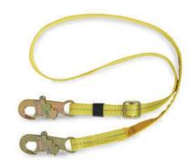
This lanyard has self-locking snaps at each end and can be adjusted from 4 to 8 ft. (1.2 to 2.4 m). Its 1-in. (25 mm) polyester web has a built-in wear indicator.
