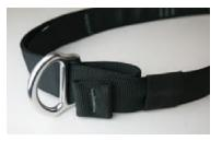
Specifically designed for performing work or rescue in or around a trench, our Class I Trench Work-Rescue Belt is loaded with features. Its AstriAlpin COBRA® buckle manufactured from 7075 aluminum alloy with a built-in stainless steel D-ring (Buckle:18 kN / 4,000 lbf MBS, D-ring: 22 kN / 5,000 lbf MBS, straight pull)—is secure yet easy to open and close while wearing gloves. Our aluminum D-ring provides a rear connection point at the back of the belt
