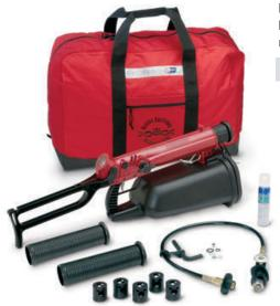
Everything you need to launch a 3 mm messenger line up to 350 ft. (107 m). The 500 ft. (152 m) Dacron $^{\circ}$  line has a tensile strength of 2.2 kN (500 lbf). Once you have the messenger line across, use it to pull across the rescue rope.
